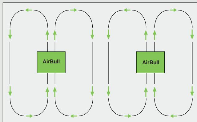
The best air purification is achieved by placing the devices so that the air can circulate in a circular motion. In this manner, the same air can be cleaned several times. In larger halls, more AirBulls should be used to ensure optimum air cleaning. The performance of AirBull can be adjusted continuously depending on the requirements (air exchange).
